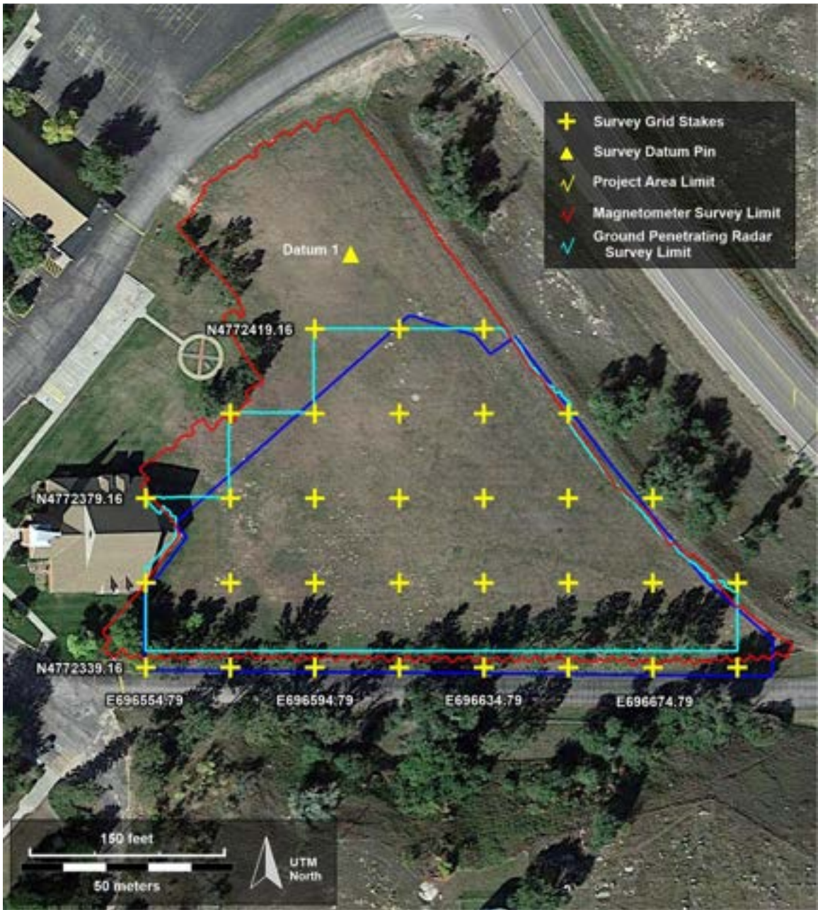
Figure 17. Map of the site survey grid and limits of the geophysical surveys relative to the project area.
