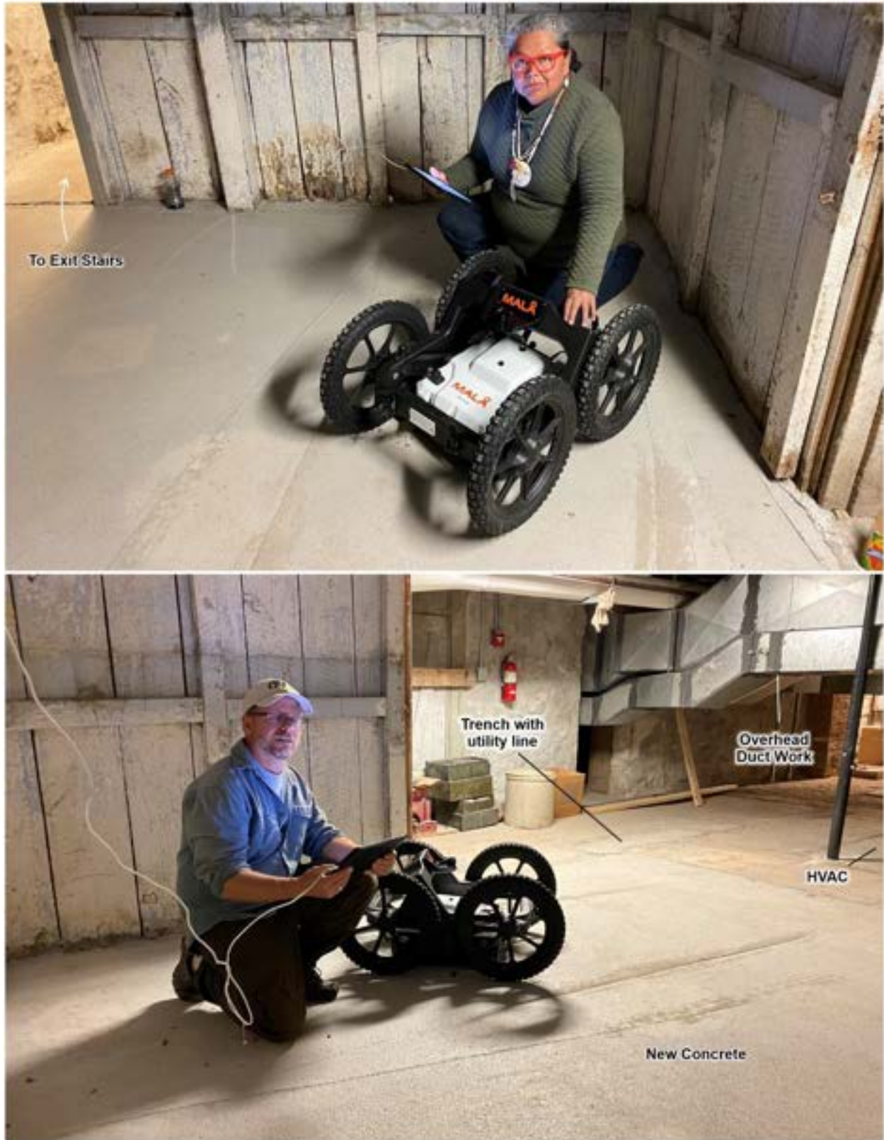
Figure 2. Authors with the Mala ground penetrating radar system used to scan the new concrete on the basement floor.
