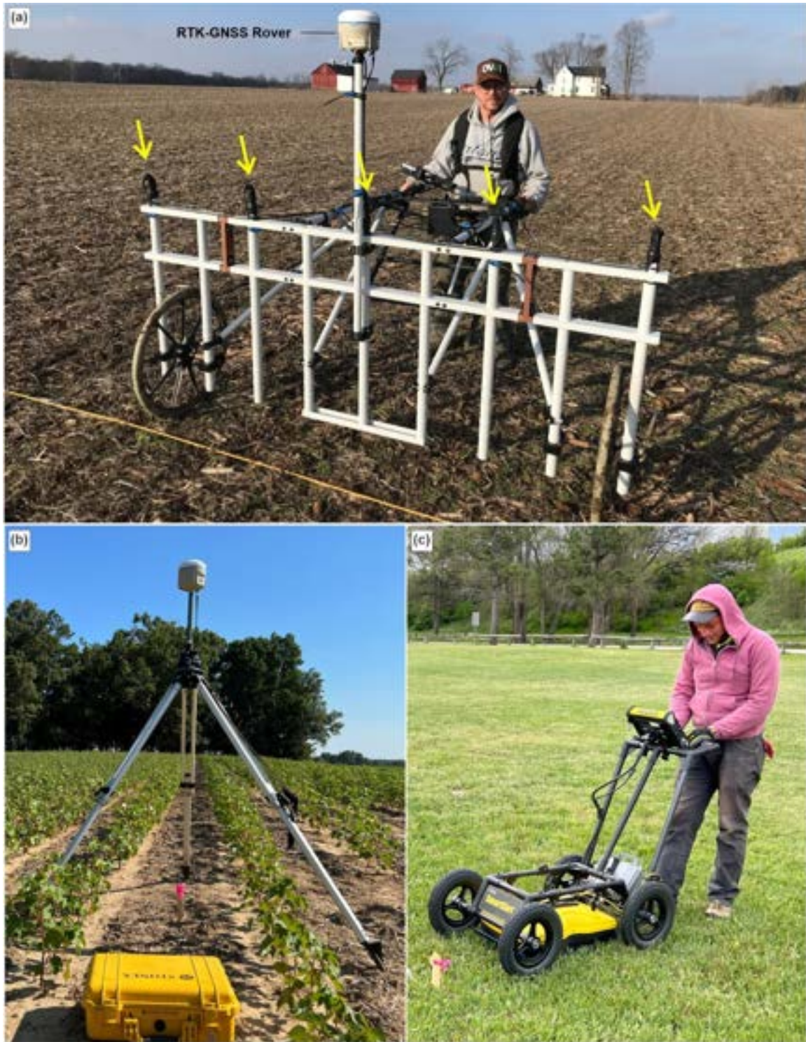
Figure 9. Geophysical survey instruments used during the survey, (a) 5-probe magnetometer system (probes indicated by yellow arrows), (b) RTK-base station paired with magnetometer system, (c) ground penetrating radar (radar image from Red Cloud).
